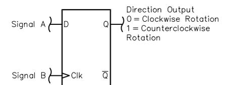
Fig 2—A rising-edge-clocked D flip-flop decodes rotation direction.
